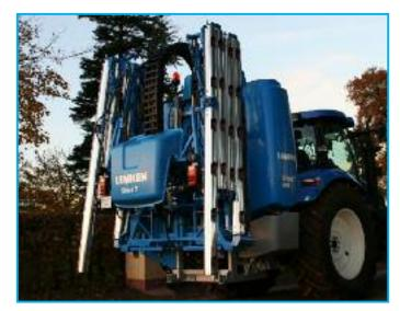
The key feature of the SectionExtend boom is the aluminium tube arm with its familiar benefits including a light, buckling resistant construction and shielded nozzle position. The fully hydraulic boom with sectional folding is vertically folded to just 2.40 metres wide behind the tank for transportation and safely stowed in its lowest position.
