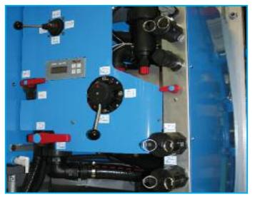
Single lever operation on the intake and pressure sides of the fittings means that almost all the functions of the sprayer can be adjusted easily using the clearly laid out, user friendly control centre on the left of the machine.
