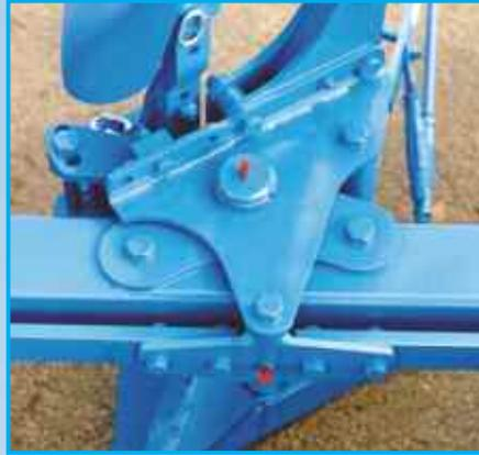
LEMKEN mount the main pivot, for each furrow, immediately beside the plough main beam. This reduces the strain on the main beam and dramatically increases its durability. Additionally, the pivot is more centrally located in relation to the pulling point of the body, which reduces the stresses and wear on the linkage and pivot. All pivot points feature wear-resistant replaceable bushes, hardened pins and lubrication points guaranteeing highest durability and long working life.
