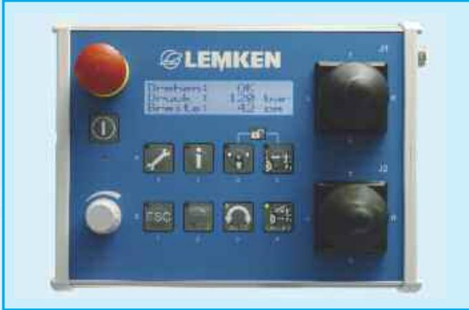
The operator selects the weight transfer to the tractor by choosing and setting a top operating pressure. A constant oil flow, via one of the tractor spool valves, allows the operating system to monitor and constantly adjust the top link to maintain the selected pressure, and transfer the optimum amount of weight to the tractor.
