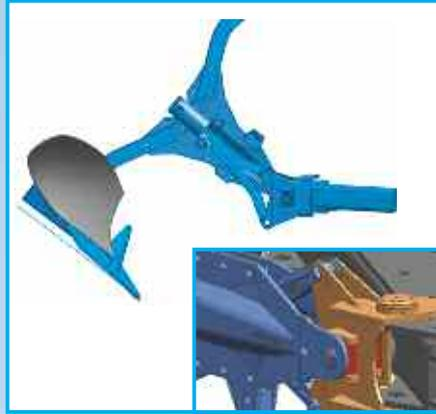
The significant advantage, of the Hydromatic system, is a firm link to the three-dimensional connection point in any position of the plough body. Thus the bodies are always kept in a stable position and cannot jump off. The innovative Hydromatic overload security element can always trip simultaneously side-ways and upwards without any problem, even when the obstacle is hit laterally.
