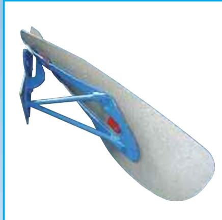
Mouldboards and slats are no longer a load bearing part of the plough body which means they serve as wear parts only. Parts can be almost completely worn out without limiting the strength of the plough body. Mouldboards, slats and shins of the DuraMaxx plough body are all hooked into a separate carrier without mounting screws or bolts.
