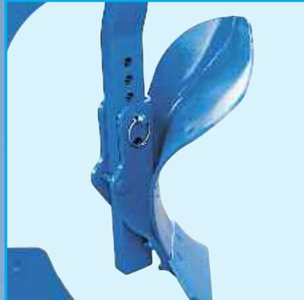
Fitting the skimmer onto a flat stalk avoids the risk of twisting. All shares and mouldboard variants can be exchanged without any problem because the frog is the common to all skimmer types. For ploughing without skimmers, loosening of two bolts allows complete removal of the skimmer arm.
