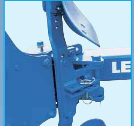
Both the VariTansanit (shearbolt) and VariTansanit T (auto-reset) are available as an option with individual quick adjustment system for the skimmer angle. This allows further fine-tuning of the skimmer performance where required.
