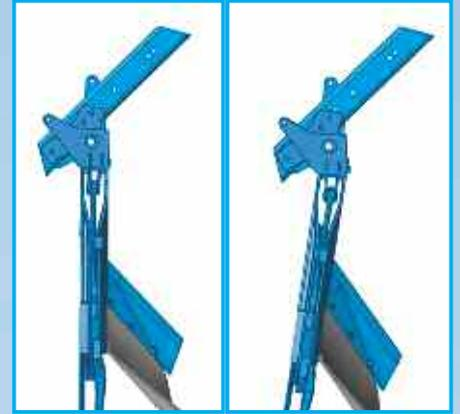
With up to 38cm upward and 20cm sideward movement, there is sufficient tripping capacity to provide continuous trouble free work even when ploughing deep. High trip forces, which are adjustable from the tractor seat, ensure the Hydromatic auto-reset system is always set to combine quality ploughing with efficient plough protection. A further benefit of the system is the lack of lubrication points – the system is maintenance-free.
