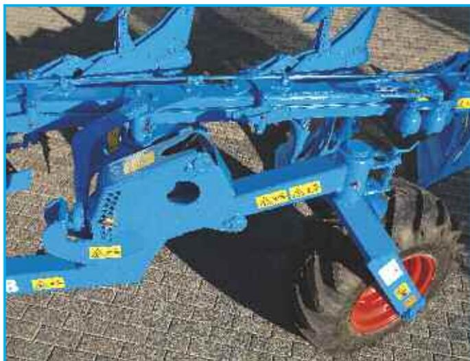
Lifting and lowering of the land wheel is automatically controlled in work by the plough's control box. A simple stop screw sets the desired ploughing depth. Road transport is safe due to the pivoting drawbar, which is hydraulically unlocked during the transport operation.
