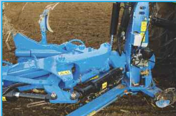
The VariTansanit is equipped with hydraulic frame swiveling, as standard, with an adjustable stop to set front furrow width. The Optiquick turnbuckle allows simple adjustment of the tractor/plough alignment using the spanner provided.
