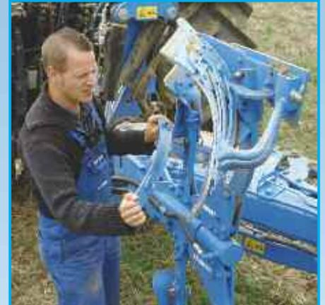
Mouldboards, slats and shins can be exchanged without tools and thus considerably faster than parts from conventional bodies. Simply removing a clip pin, allows the shin to be removed which, itself, acts as a locking device for the slats or solid mouldboard. The point is fixed with a single screw which additionally decreases the replacement time required. Measurements have resulted in set-up times that are 80% lower than that conventional plough bodies.
